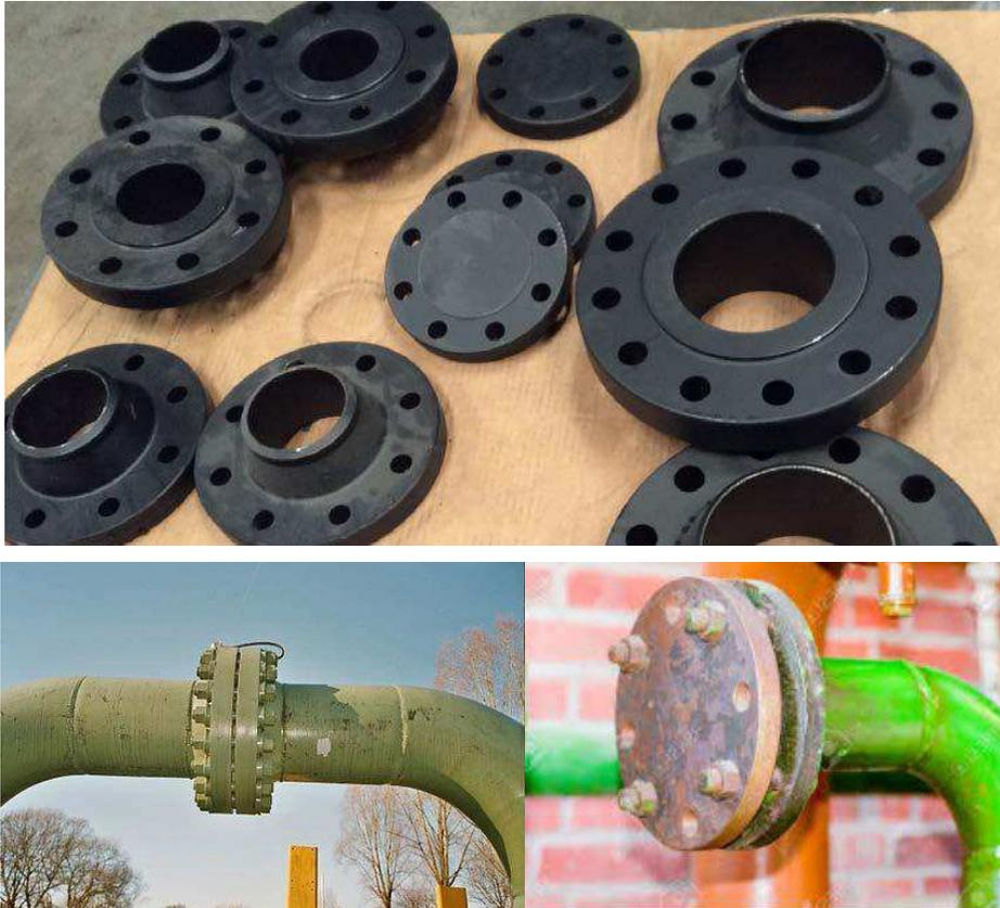
12. Flanges are also made with various differentiators including facings, number of bolt holes, and pressure classes.<sup>1</sup> Flanges may be manufactured in specific dimensions provided by the customer or they may be made according to published specifications. Finally, flanges can be manufactured using various materials. Carbon steel, which is strong, durable, and relatively low in cost, is the most commonly used material for flanges.
