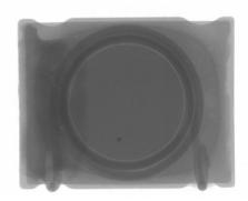
The following photographs show the optical cross-section and x-ray image of the coil wound about the core of the Accused Inductors:
