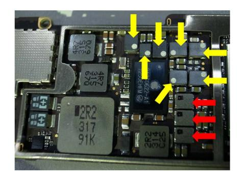
10. The Accused Inductors have enhanced inductance. On information and belief, the Accused Inductors exhibit an enhanced inductance through adjusting the thickness of the magnetic-resin layer. *See* '390 patent col 3:31-32; col. 4:13-29.
