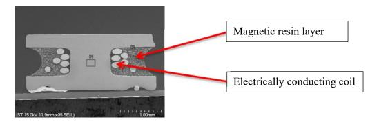
14. The magnetic resin layer contained in the Accused Inductors contains a magnetic powder dispersed in a polymer resin. The spectrum below indicates that the magnetic resin layer contains approximately 35% iron (Fe), a magnetic substance, and approximately 51% carbon (C), that is used for the polymer resin.
