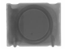
The following photographs show the optical cross-section and x-ray image of the coil wound about the core of the Accused Inductors:
