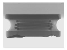
21. The inductors used in Defendant's iPad 4 tablet computers were made using a method that includes forming a magnetic resin layer by compression molding to embed at least a portion of an outer periphery of said electrically conducting coil. On information and belief, the resin layer is compression-molded.
